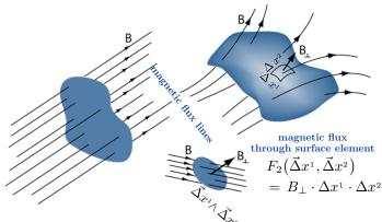
The density and orientation of magnetic field flux lines are encoded in a differential 2-form whose integral over a given surface is proportional to the total magnetic flux through that surface. (Graphics adapted from [Hyperphysics].)
