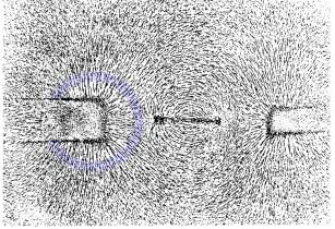
From Faraday's *Diary of experimental investigation*, vol VI, entry from 11th Dec. 1851, as reproduced in [Martin09]; the colored arc is our addition, for ease of comparison with the schematics on the right.
